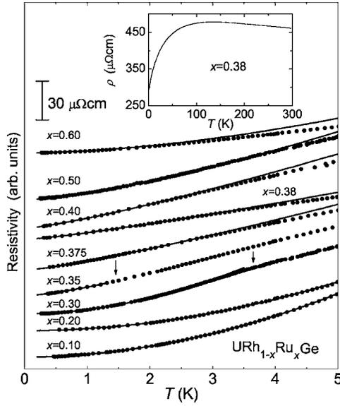
FIG. 3. Resistivity of  $\text{URh}_{1-x}\text{Ru}_x\text{Ge}$  for  $0.10 \leq x \leq 0.60$ . The bar gives the absolute scale. The arrows for  $x=0.30$  and  $0.35$  indicate  $T_C$  obtained from additional data sets. The solid lines are fits to  $\rho(T) = \rho_0 + AT^n$ . For  $x \leq 0.3$ ,  $n = 2.0 \pm 0.1$ . For  $x_{cr} = 0.38$ ,  $n = 1.2$  is minimum. Inset: Resistivity for  $x=0.38$  up to 300 K.
