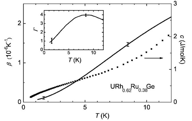
FIG. 4. Coefficient of volume thermal expansion  $\beta(T)$  (solid line) and specific heat  $c(T)$  ( $\bullet$ ) of  $\text{URh}_{0.62}\text{Ru}_{0.38}\text{Ge}$ . Inset: Grüneisen ratio  $\Gamma$  as a function of  $T$ .
