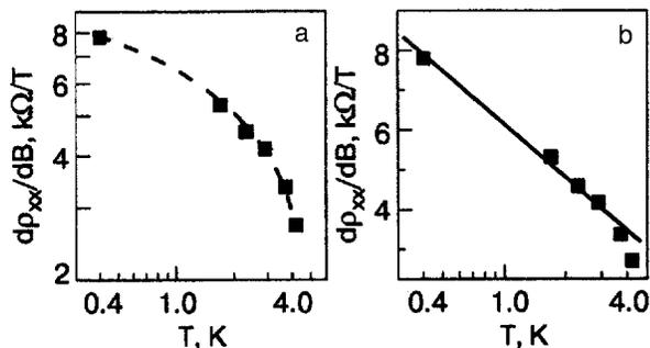
FIG. 2. The first derivative  $d\rho_{xx}/dB$  as a function of temperature in the vicinity of the low-field critical point in log-log scale (a) and linear-log scale (b). The dashed line in panel “a” is a guide to the eye.
