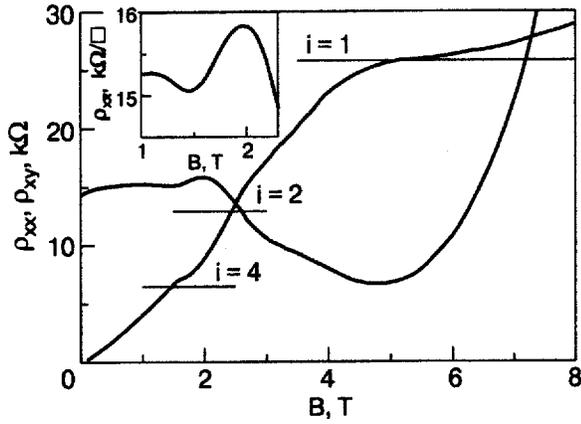
FIG. 4. Longitudinal and Hall resistivities as functions of magnetic field for sample B at  $T=0.4$  K.
