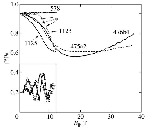
**Fig. 2.** Magnetoresistances of different samples in a parallel magnetic field at  $T = 1.6 \text{ K}$ . The asterisk indicates the local features in the magnetoresistance of samples 475a2 and 476b4. The inset shows the magnetoresistances of samples 475a2 and 476b4 after subtracting the monotonic component.
