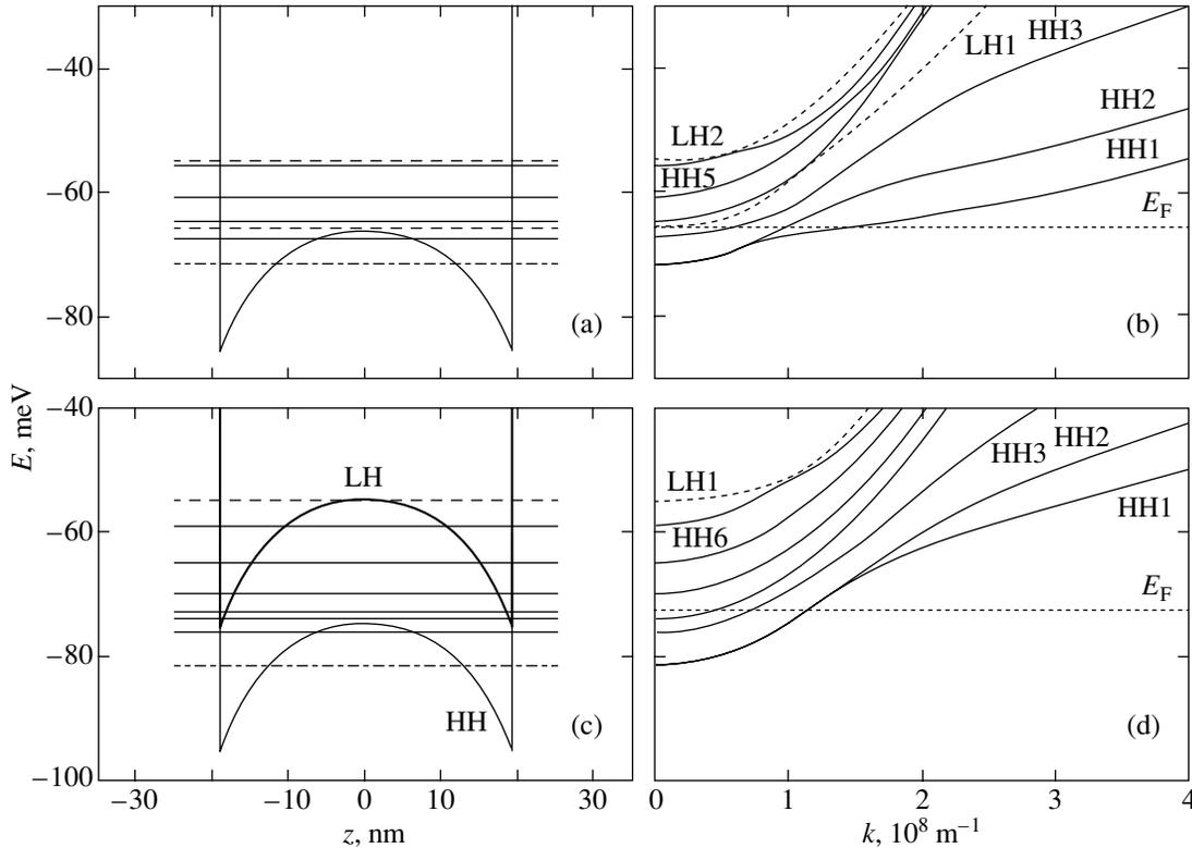
**Fig. 4.** Calculated valence band structure for sample 475a2. The energy increases deep into the valence band. The potential profiles and energy levels are calculated (a) without regard for the strain and (c) at the strain parameter  $\zeta = 10$  meV. The structures of the corresponding subbands and the Fermi levels are calculated (b) without regard for the strain and (d) at the strain parameter  $\zeta = 10$  meV.
