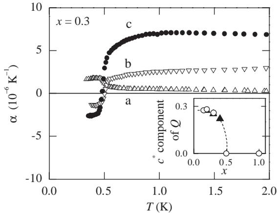
Fig. 1. Temperature dependence of the linear thermal expansion coefficients  $\alpha_i$  (with  $i = \mathbf{a}, \mathbf{b}, \mathbf{c}$ ) of  $\text{CeCu}_{5.7}\text{Au}_{0.3}$ . The inset shows the reciprocal  $\mathbf{c}^*$ -axis component of the magnetic ordering wave vector  $\mathbf{Q}$ .
