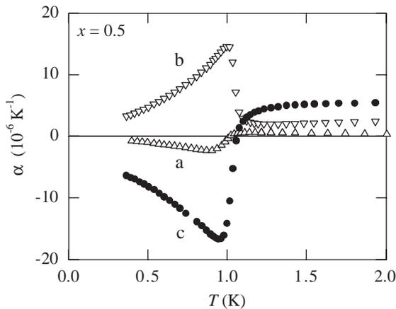
Fig. 2. Temperature dependence of the linear thermal expansion coefficients of  $\text{CeCu}_{5.5}\text{Au}_{0.5}$ .
