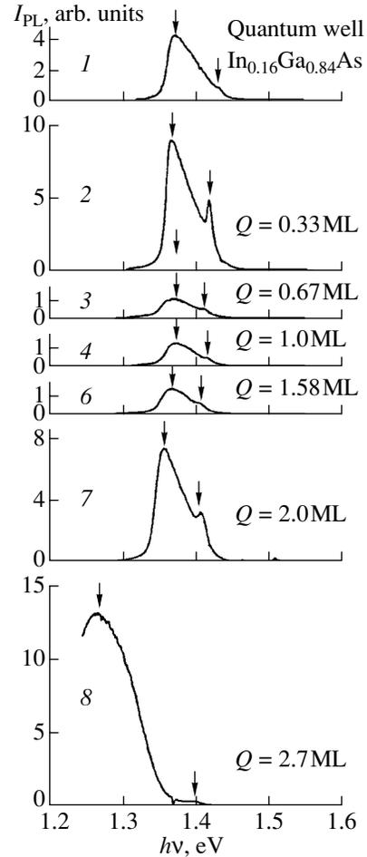
**Fig. 6.** Photoluminescence spectra of the investigated structures, which differ in the nominal thickness  $Q$  of the InAs layers. The scale on the axis of the PL intensity  $I_{PL}$  is identical for all drawings. Drawings are numbered according to sample numbers in the table.  $T = 77$  K.
