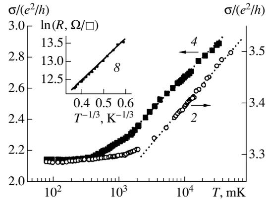
**Fig. 4.** Conductivity  $\sigma$  for samples 2 and 4 in units of the lowest metallic conductivity  $e^2/h$  at low temperatures. The dependence of resistance  $R$  on the temperature  $T$  for sample 8 in the coordinates corresponding to the Mott law is in the inset. Curves are numbered according to sample numbers in the table.
