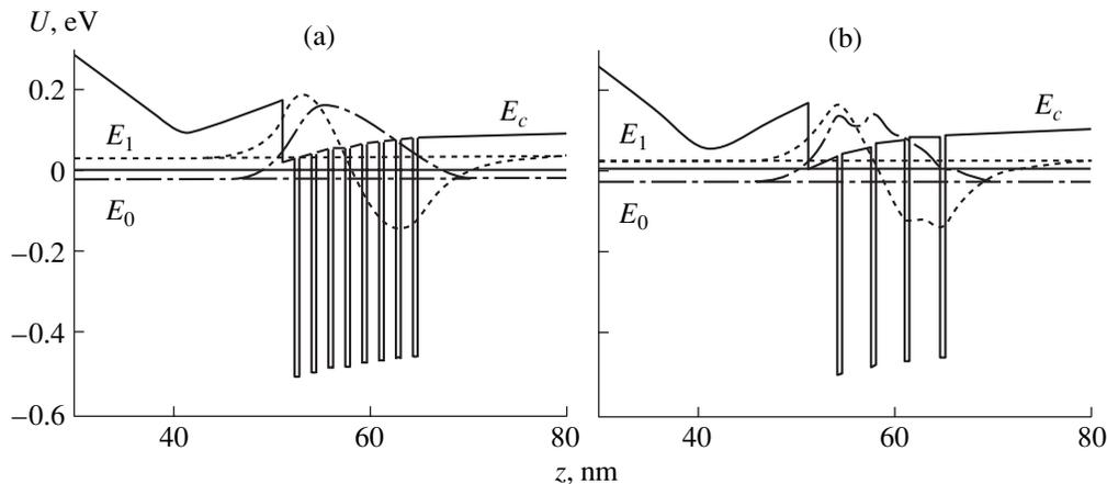
**Fig. 8.** Calculated profile of the conduction-band bottom ( $E_c$ ), the position of the lower electron levels  $E_0$  (dash-and-dot line) and  $E_1$  (dashed line), as well as the profile of corresponding wave functions for samples (a) 4 and (b) 7. The letter  $z$  denotes the distance from the sample surface. The Fermi level is denoted by a solid horizontal line.
