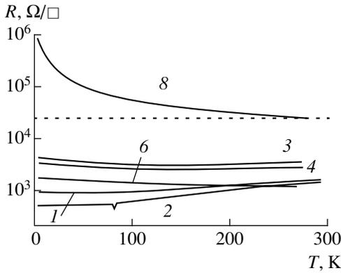
**Fig. 3.** Temperature dependences of resistance  $R$  per area for samples 1–6 with short-period superlattices and sample 8 with QD layers. A horizontal dotted straight line corresponds to the  $h/e^2$  value. Curves are numbered according to sample numbers in the table.
