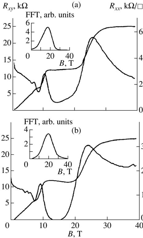
**Fig. 5.** Transverse magnetoresistance  $R_{xx}$  and Hall resistance  $R_{xy}$  of samples (a) 4 and (b) 6 at  $T = 4.2$  K. Curves are numbered according to sample numbers in the table. The relevant Fourier spectra are shown in inset.
