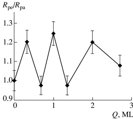
**Fig. 9.** Ratio of resistance in the  $[\bar{1}10]$  direction ( $R_{pe}$ ) to the resistance in the  $[110]$  direction ( $R_{pa}$ ) as a function of the thickness of the InAs layers ( $Q$ ). The value  $Q = 0$  ML corresponds to sample 1.
