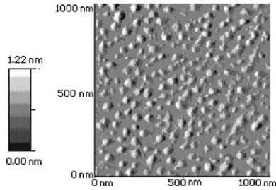
Fig. 1. Typical AFM image of an InAs QD layer surface after selective etching.
