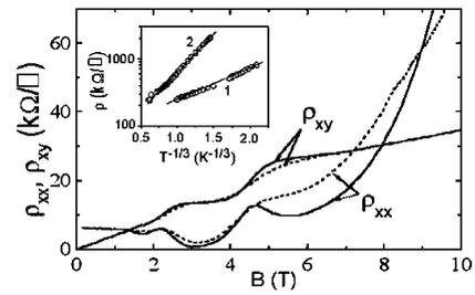
Fig. 3. Oscillations of the magnetoresistivity  $\rho_{xx}$  and the Hall resistivity  $\rho_{xy}$  at temperatures  $T = 1.7$  K (solid lines) and  $T = 4.2$  K (dashed lines) for sample 3. Inset show the temperature dependence of resistivity for samples 1 and 2.
