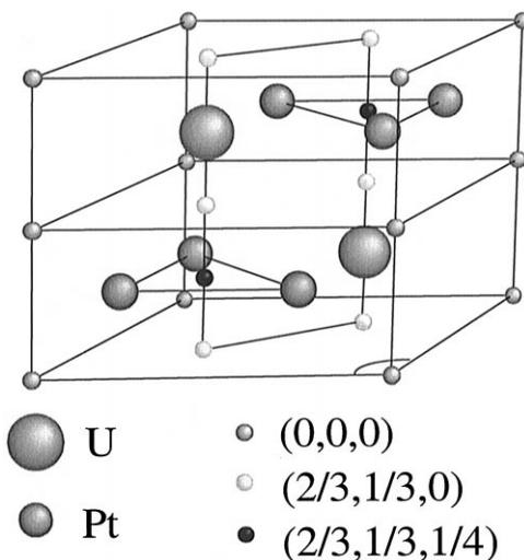
Fig. 4. The crystallographic unit cell of  $UPt_3$  (space group  $P6_3/mmc$ ). The axial symmetric sites (0,0,0),  $(\frac{2}{3}, \frac{1}{3}, 0)$  and  $(\frac{2}{3}, \frac{1}{3}, \frac{1}{4})$  are indicated.
