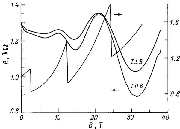
FIG. 9. Dependence of the resistance of sample 2 on the magnetic induction parallel to the  $\delta$  layer for two orientations of the current through the sample relative to the magnetic field and ratio of the calculated density of states at the Fermi level  $g(B)$  to the density of states in the absence of a magnetic field  $g(0)$ .
