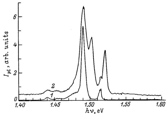
FIG. 6. Isolated parts of the photoluminescence spectra of the control sample without a  $\delta$  layer (1) and sample 5 (2) at  $T=4.2$  K. The photoluminescence intensities are the same as in Fig. 5.
