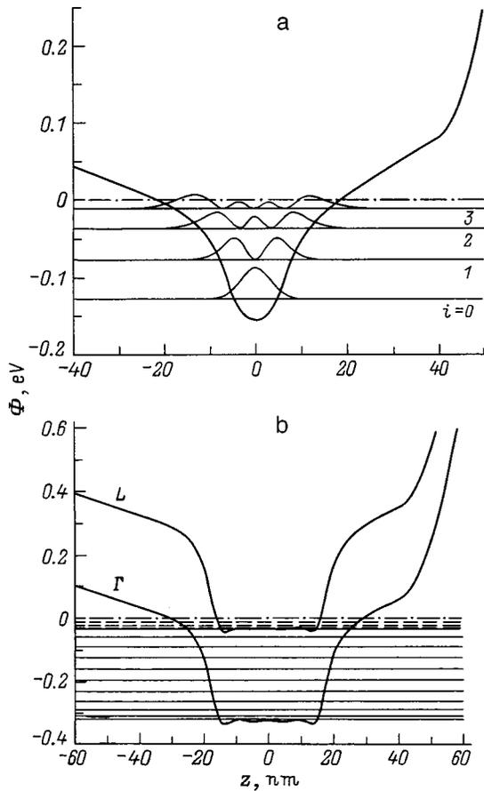
FIG. 4. Band diagrams for samples 5 (a) and 6 (b). The energy is measured relative to the Fermi level (dot-dashed line). The free surface of the samples is located at  $z = 60$  nm. The squares of the electronic wave functions in the subbands are also shown for sample 5. The energy levels at the  $L$  point in sample 6 are indicated by dashed lines.
