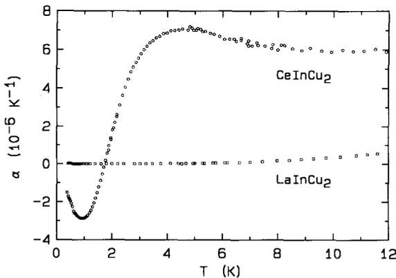
Fig. 1. Coefficients of linear thermal expansion of polycrystalline CeInCu<sub>2</sub> (○) and LaInCu<sub>2</sub> (□).
