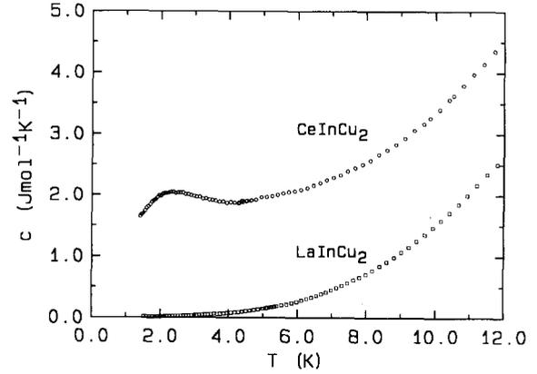
Fig. 2. Specific heat of polycrystalline CeInCu<sub>2</sub> (○) and LaInCu<sub>2</sub> (□) after ref. [1].
