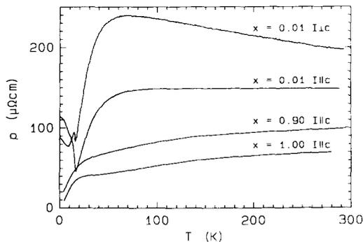
Fig. 2. Temperature dependence of the electrical resistivity of single crystalline  $U_{1-x}Ce_xRu_2Si_2$  for  $x = 0.01, 0.90$  and  $1.00$  and for current directions as indicated.
