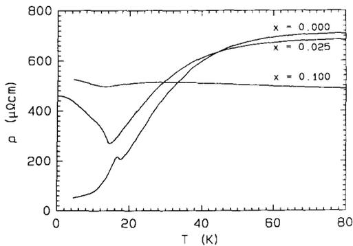
Fig. 1. Temperature dependence of the electrical resistivity of polycrystalline  $U_{1-x}Ce_xRu_2Si_2$  for  $x = 0.00, 0.025$  and  $0.10$ .
