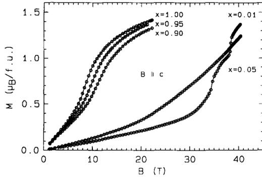
Fig. 4. High field magnetization ( $B \parallel c$ ) of single crystalline  $U_{1-x}Ce_xRu_2Si_2$  for  $x = 1.00, 0.95, 0.90$  and  $0.05$  at  $T = 4.2$  K and for  $x = 0.01$  at  $T = 1.5$  K.
