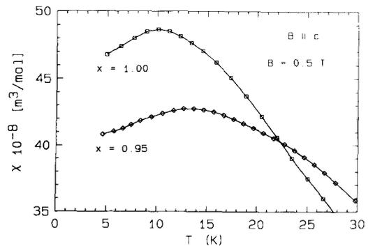
Fig. 3. Magnetic susceptibility ( $B = 0.5$  T,  $B \parallel c$ ) of single crystalline  $U_{1-x}Ce_xRu_2Si_2$  for  $x = 1.00$  and  $x = 0.95$ .
