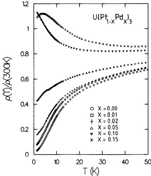
Fig. 3. Reduced resistivity,  $\rho(T)/\rho(300\text{ K})$ , of polycrystalline  $U(\text{Pt}_{1-x}\text{Pd}_x)_3$  samples, for  $x = 0.00$  ( $\circ$ ),  $0.01$  ( $\square$ ),  $0.02$  ( $+$ ),  $0.05$  ( $\triangle$ ),  $0.10$  ( $\nabla$ ) and  $0.15$  ( $\times$ ).
