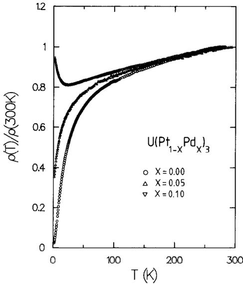
Fig. 1. Reduced resistivity,  $\rho(T)/\rho(300\text{ K})$ , of monocrystalline  $U(\text{Pt}_{1-x}\text{Pd}_x)_3$  whiskers, for  $x = 0.00$  ( $\circ$ ),  $0.05$  ( $\Delta$ ) and  $0.10$  ( $\nabla$ ). The current is applied along the  $c$ -axis.
