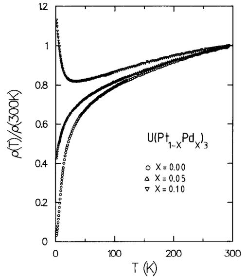
Fig. 2. Reduced resistivity,  $\rho(T)/\rho(300\text{ K})$ , of polycrystalline  $U(\text{Pt}_{1-x}\text{Pd}_x)_3$  samples, for  $x = 0.00$  ( $\circ$ ),  $0.05$  ( $\Delta$ ) and  $0.10$  ( $\nabla$ ).
