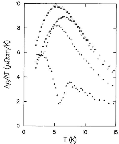
Fig. 4. Temperature derivative of the resistivity,  $\Delta\rho/\Delta T$ , of polycrystalline  $U(\text{Pt}_{1-x}\text{Pd}_x)_3$  samples, for  $x = 0.00$  ( $\circ$ ),  $0.01$  ( $\square$ ),  $0.02$  ( $+$ ) and  $0.05$  ( $\triangle$ ).
