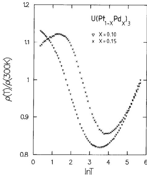
Fig. 5. Reduced resistivity,  $\rho(T)/\rho(300\text{ K})$ , versus  $\ln T$  of polycrystalline  $U(\text{Pt}_{1-x}\text{Pd}_x)_3$  samples, for  $x=0.10$  ( $\nabla$ ) and  $0.15$  ( $\times$ ).
